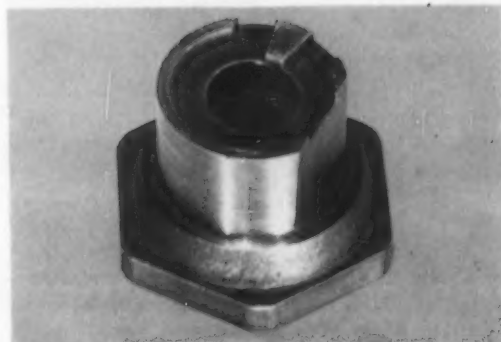
Right: MORE than 1/2 hour of machining time is saved by investment casting this alloy steel knob.
